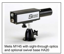
**Lenses:** The pyrometer is sensitive to infrared radiation in an area called cone of vision. This area has to be kept free from any intervening objects. The infrared energy radiated by the hot gas is centered via focusable or fixed focus lenses directly on the detector. The focusing feature allows control of the cone of vision and offers the possibility to measure either a small spot (focused) or the average of a bigger spot (out of focus).
