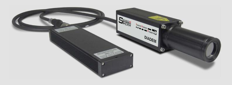
Digital transfer standard pyrometer for high-precision inspection of calibration sources
