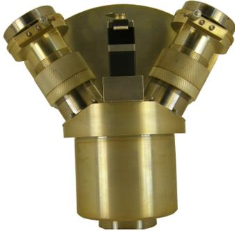
The Resonance Ltd. vacuum monochromator and spectrometer uses standard connections to allow simple integration into most systems. The f/4.2 grating is a type 4 for minimal aberrations. It is designed to allow easy interchangeability between being a monochromator with servo-controlled drive and a CCD-based spectrometer. It's supplied with LabView-based codes and drivers for integration into user software.
