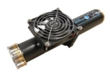
Resonance Ltd. UV Optically Thin Molecular sources are designed to be reliable and maintenance free compact sources of UV emissions with an operating life in excess of 500 hours. Suitable for molecular absorption and fluorescence measurements.
