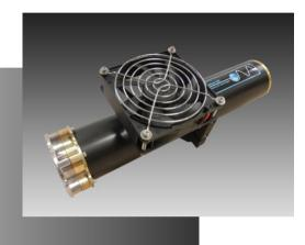
Resonance Ltd. RF Powered Line sources are designed to be reliable and maintenance free compact power sources of emissions with an operating life in excess of 4000 hours. Line sources are sealed RF excited with a window in an EMI shielded enclosure. The lamp mounts to a 2.75 inch or larger CF type flange. The lamp assembly has an integral RF exciter which is powered by a small wall plug power supply.
