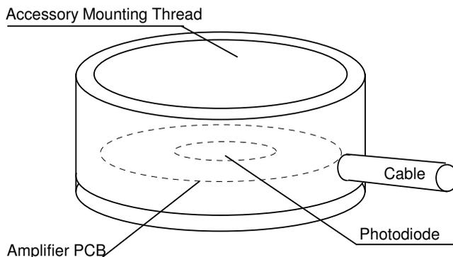
The DET203QR laboratory detector comprises of a aluminium housing, photodiode and PCB assembly.
