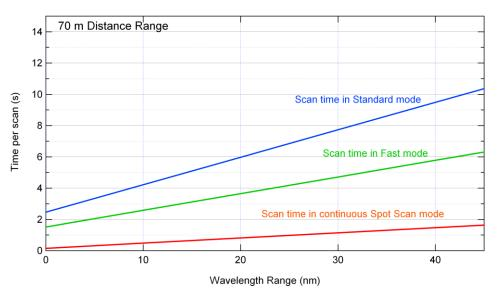
Time per scan vs. scan wavelength range for 70 m scans in standard operating, fast scanning and continuous spot scanning modes.
