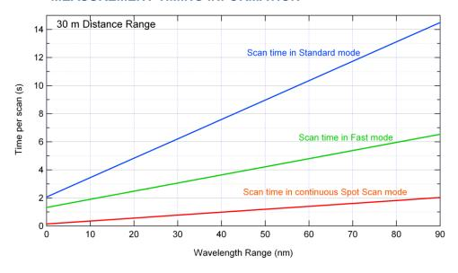
Time per scan vs. scan wavelength range for 30 m scans in standard operating, fast scanning and continuous spot scanning modes.
