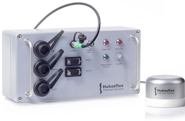
Figure 3 the complete STPSYS05 system. The STP05 sensor, also available as a 'sensor only', is meant for measuring the thermal conductivity of materials at their interface. It is equipped with a heater (line source), a temperature difference sensor (thermopile) and a temperature sensor (thermistor).
