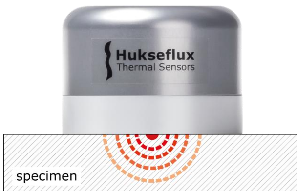
Figure 1 STP05 thermal properties sensor, with a schematic view of the cylindrical thermal field (isotherms). STP05 is conveniently placed at the surface of the specimen, and the heat from STP05's line-source penetrates several millimetres into the material; the measurement is representative for this entire volume.
