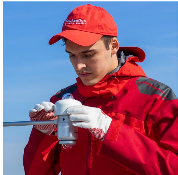
Figure 5 using SRA30 albedometer is easy; the instrument is composed of AMF03 and two SR30-M2-D1 pyranometers
