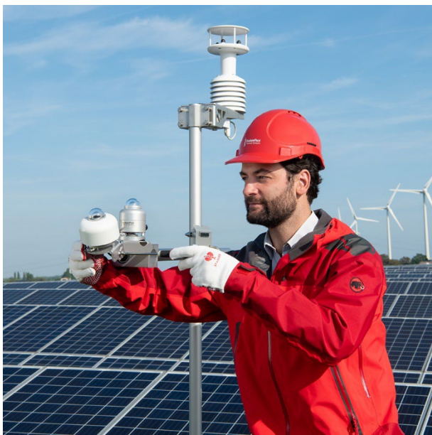
Figure 2 Two SR300-D1 pyranometers, one tilted for Plane of Array (POA) measurement, and another mounted horizontally for Global Horizontal Irradiance (GHI) measurement.
