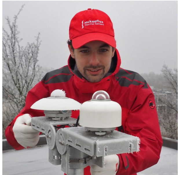
Figure 3 Heated to counter frost and dew deposition: clear difference between a non-heated pyranometer (back) and SR30 with RVH™ technology (front)
