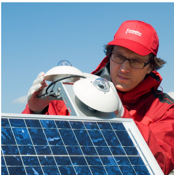
Figure 2 PV system performance monitoring pyranometers
