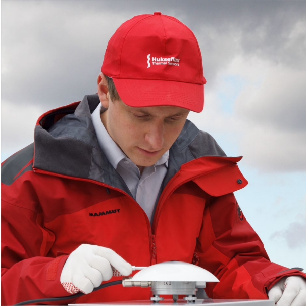
Figure 3 IR20 pyrgometer being prepared for application
