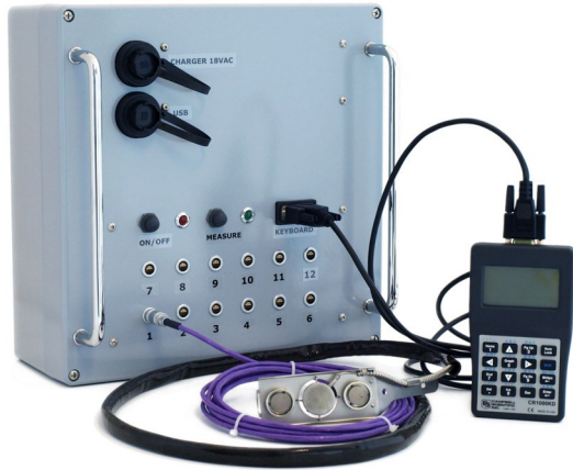
Figure 4 the ALUSYS measuring system, for trend - monitoring and comparative surveys of heat fluxes and surface temperature on industrial installations. Connected is one HF01 sensor, as well as the Keyboard Display.
