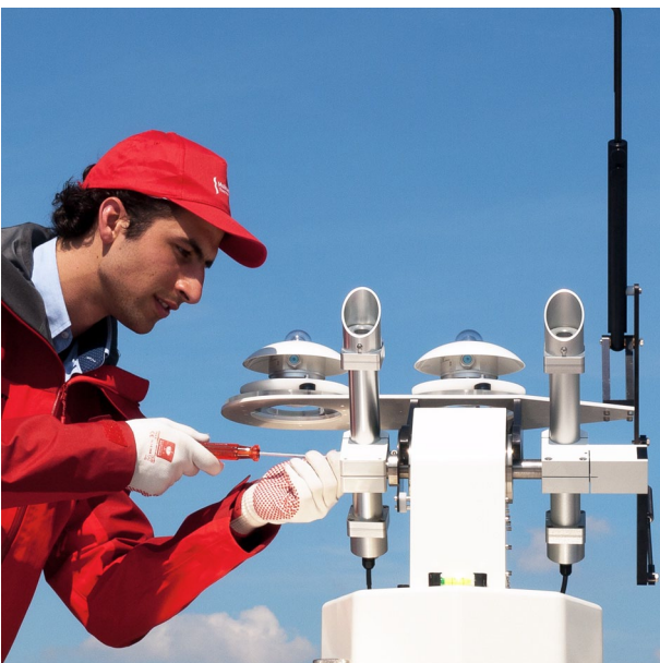
Figure 3 Two DR01s in use in tracker-mounted operation
