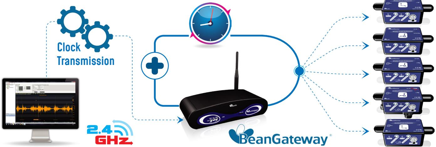
TimeSync function brings time-synchronization over the Wireless IIOT Sensors ( $\pm 2.5\text{ms}$  of accuracy between each Wireless IIOT Sensors) and contributes to enhance user experience about correlation of remote sensing data and modal analysis
