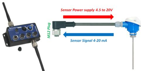
The sensor is directly powered by a high accuracy and adjustable DC/DC converter integrated inside the device. The excitation voltage is remotely configurable through the **BeanScope®** (4.5 to 20V).
