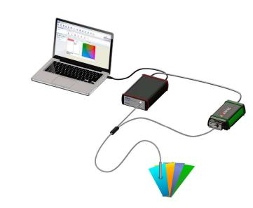
standard tile is needed for calibration. Color measurements may be applied to a variety of industrial applications such as color of textile, paper, fruit, wine, and bird feathers. Avantes has developed a variety of custom probes to meet the specific demands of the color measurement application. Color measurements are manifested in the L\*a\*b\* color model which includes parameters for brightness and hue.
