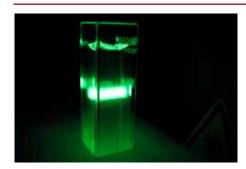
In spectroscopy fluorescence is one of the more challenging setups, due to the low fluorescent emission (about 3% of the excitation energy). The AvaSpec-2048L gives the highest sensitivity and the AvaLight-LED series provides excitation at the requested wavelength.
